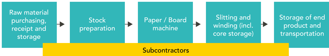
Figure 4 - Flow Chart for Papermaking Process
